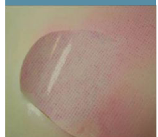
Figure 18. Membrane surface after dye test
